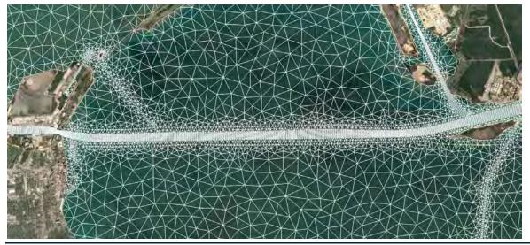
Figure 3.2: Computational mesh for the MIKE sedimentation model showing the grid cells in the channel
